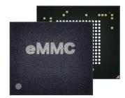
EH150-eMMC serves as the ideal storage solution for a wide range of industrial applications, including embedded systems, factory automation, networking, transportation, aerospace and defense, surveillance, medical equipment, and more. Its compact BGA package sizes and minimal power consumption render eMMC an affordable and efficient memory solution for mobile and embedded products.
