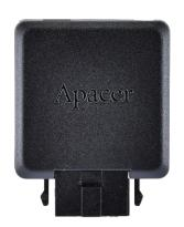
In terms of flash management, UV110-UFM3 adopts the latest page mapping file translation layer and comes with various implementations including power saving modes, wear leveling, flash block management, power failure management, S.M.A.R.T., Hyper Cache technology and SMART Read Refresh™. With cost-effective design, better performance and increased reliability, UV110-UFM3 is well suited for embedded flash storage applications offering new and expanded functionality.
