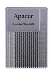
PV19E-25W offers a wide range of capacities up to 25,600 GB and delivers outstanding performance up to 7,460 MB/s (for sequential read) and 7,100 MB/s (for sequential write) based on eTLC NAND flash with the DDR4. Moreover, the power consumption of U.3 (15mm) SSD is much lower than traditional hard drives, making it the best embedded solution for new platforms.
