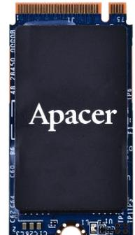
Utilizing 3D NAND technology for higher capacities up to 1TB and offering superior power efficiency compared to 2D NAND, PT25P-M242 is equipped with advanced features to enhance SSD performance and reliability. It incorporates an LDPC (Low Density Parity Check) ECC engine to extend SSD endurance and enhance data reliability.
