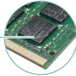
● Apacer DRAM module with conformal coating
